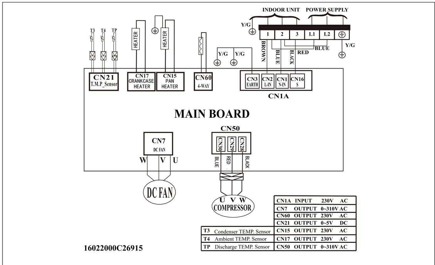
Figure 37. 09K, 12K and 18K - 208/230VAC Outdoor Unit Wiring Diagram
