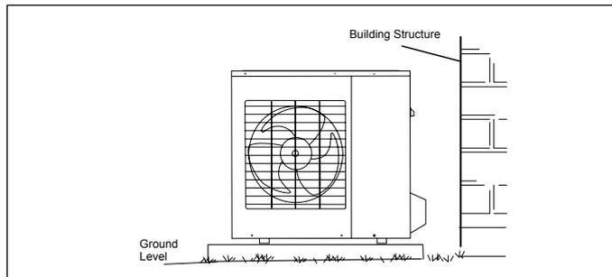
**Figure 17. Install Unit Level**
