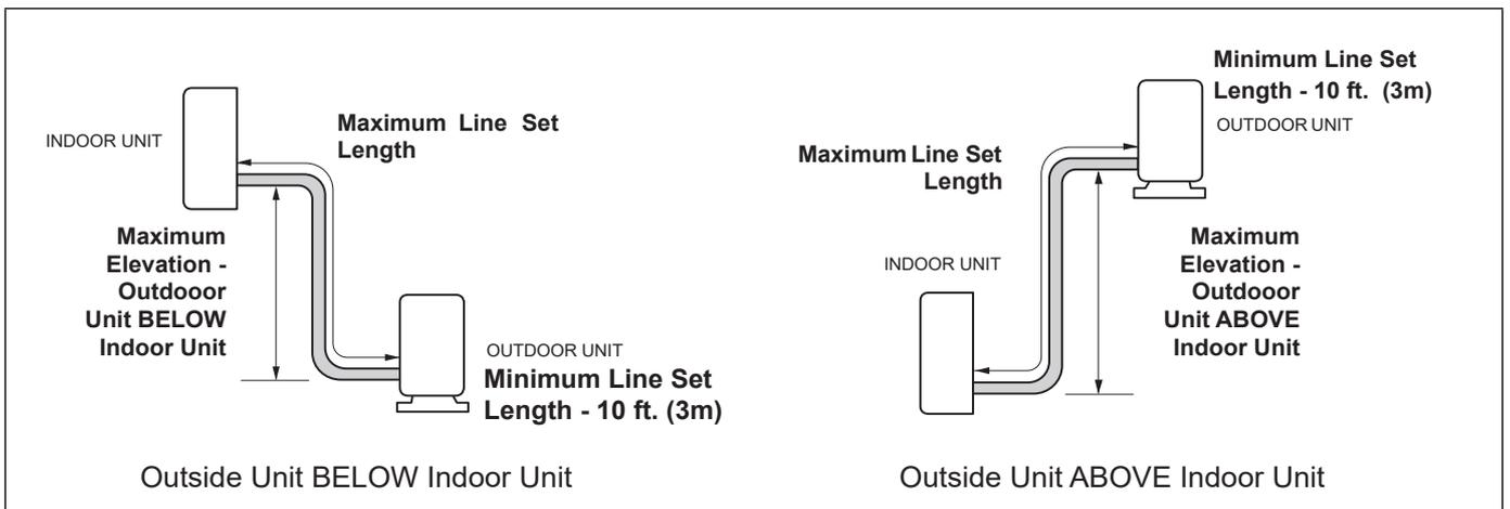
**Figure 30. Indoor and Outdoor Unit Elevation Relationships**
