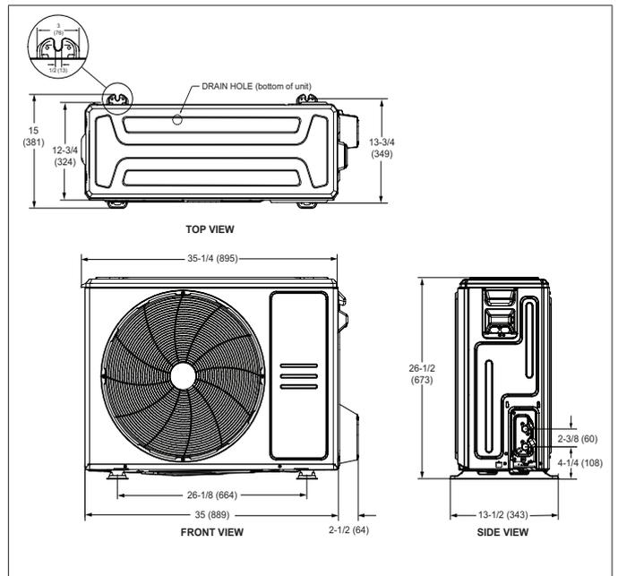
Figure 4. 24K Outdoor Unit Dimensions - Inches (mm)
