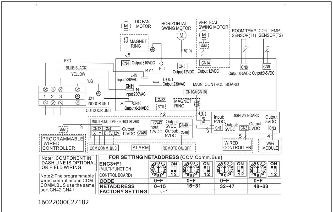
Figure 35. MWHB 24K 208/230VAC Indoor Unit Wiring Diagram
