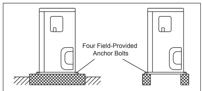
**Figure 25. Securing Outdoor Unit to Rails**
