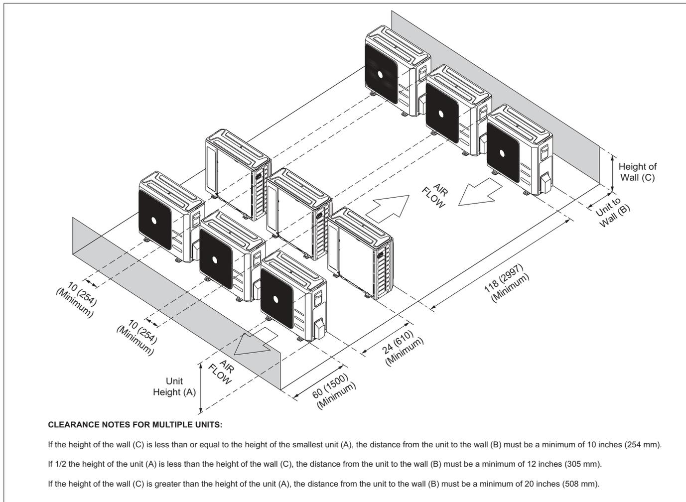
Figure 10. Multiple Outdoor Unit Clearances - Inches (mm)
