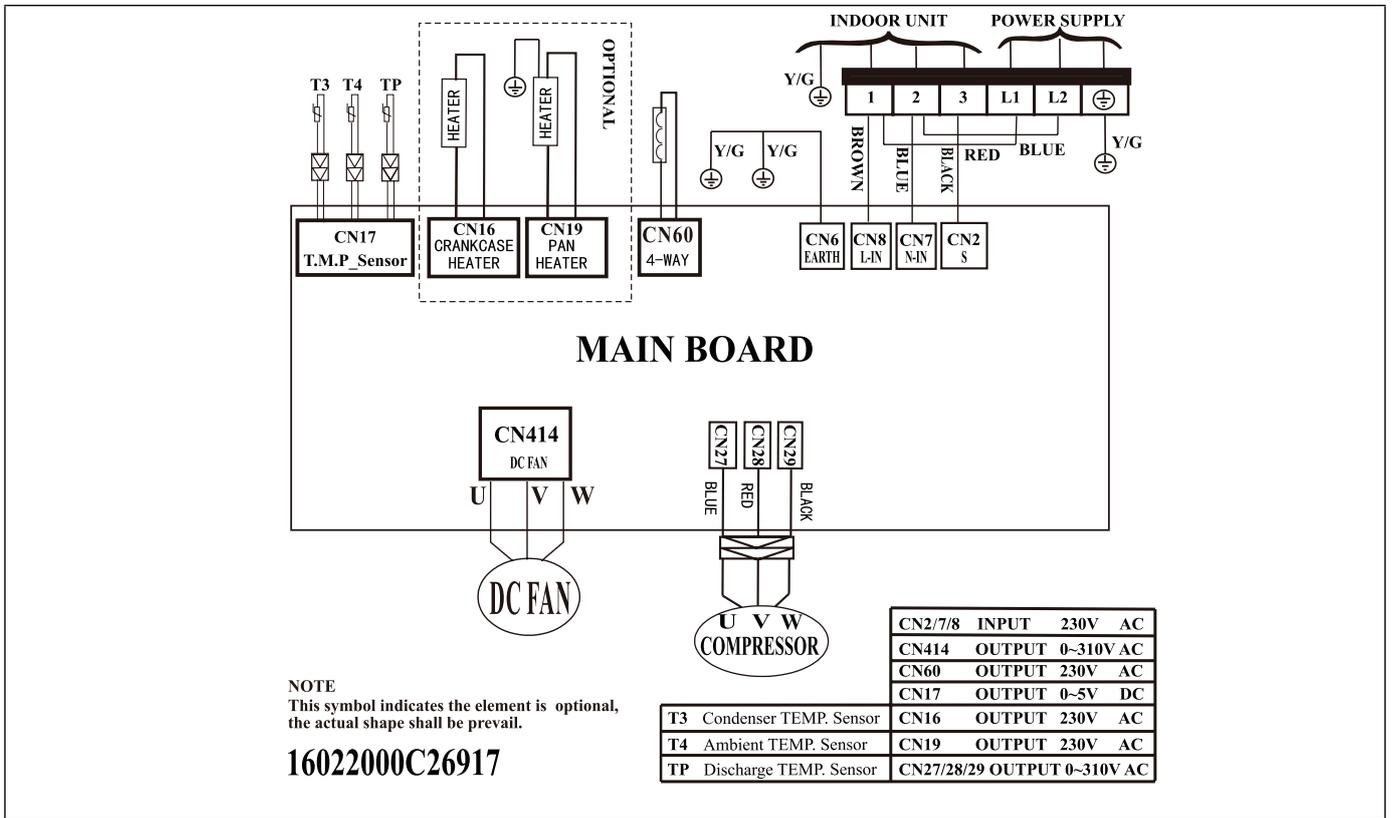
Figure 38. MHB 24K - 208/230VAC Outdoor Unit Wiring Diagram
