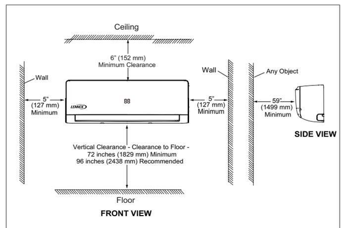
Figure 9. Indoor Unit Clearances - Inches (mm)
