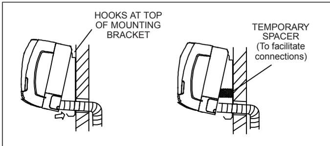
Figure 14. Secure Unit to Wall Mounting Plate
