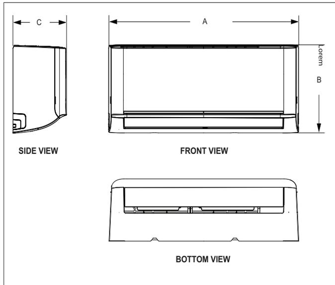
Figure 5. Indoor Unit Dimensions - Inches (mm)
