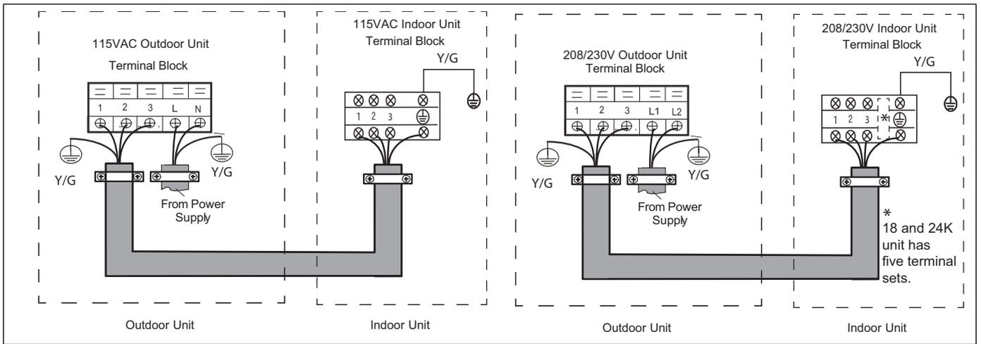
**Figure 32. Single Zone Wiring**
