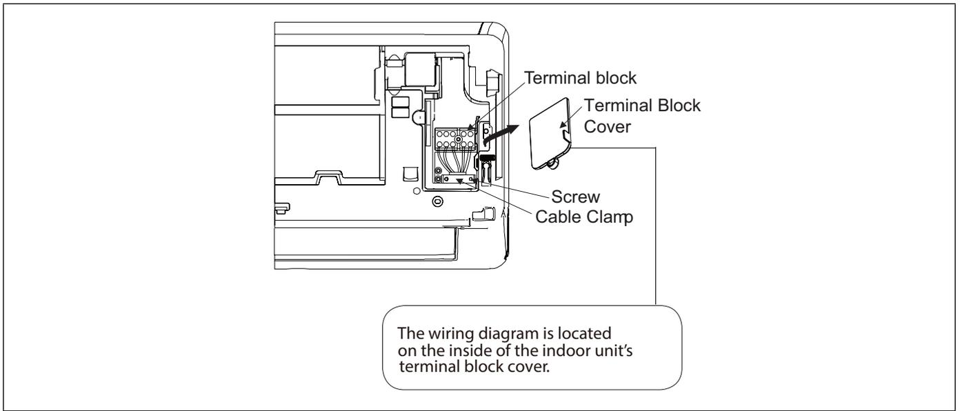
**Figure 31. Indoor Unit Terminal Block**
