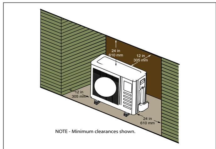
**Figure 20. Unit installed in Alcove**
