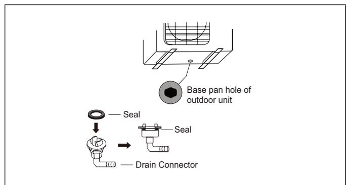
Figure 16. Installing Drain Connector and Seal
