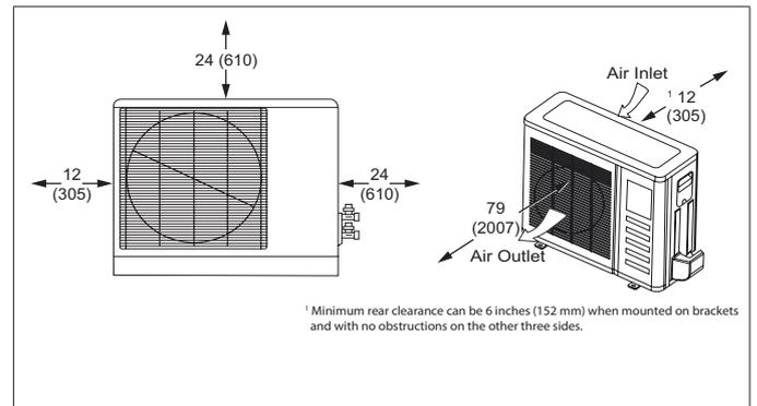
Figure 8. Outdoor Unit Clearances - Inches (mm)
