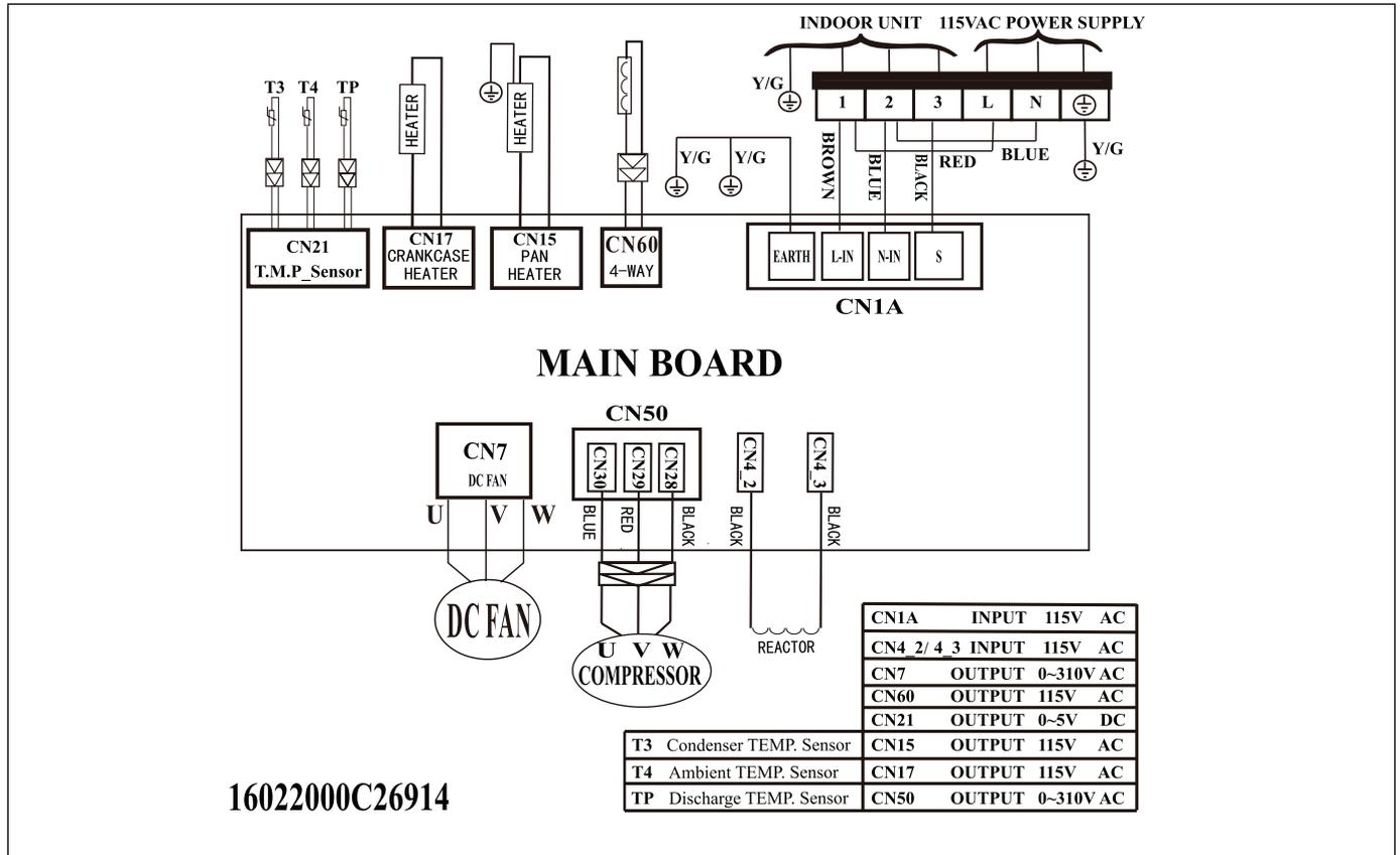
Figure 36. MHB 9K and 12K - 115VAC Outdoor Unit Wiring Diagram
