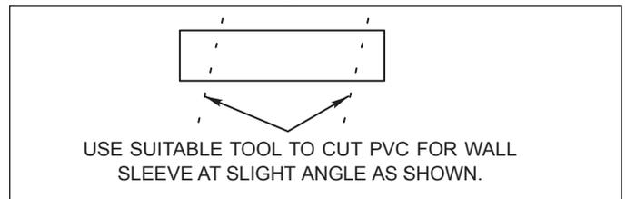
**Figure 13. PVC Wall Sleeve Installation**
