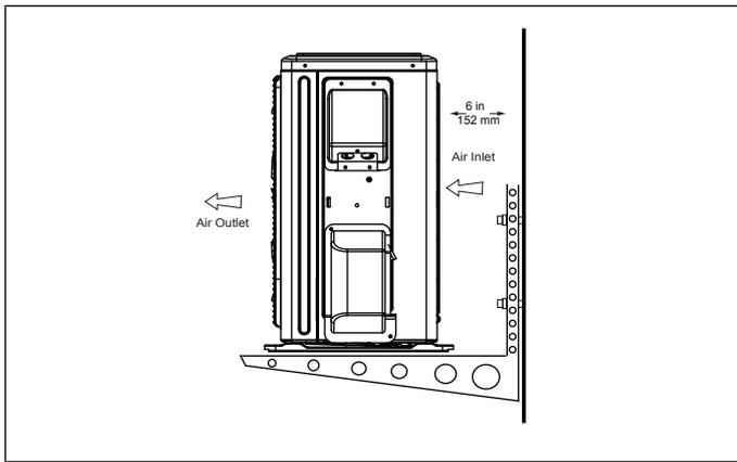
**Figure 26. Securing Outdoor Unit to Brackets**
