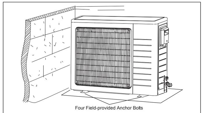
**Figure 24. Securing Outdoor Unit to Slab**
