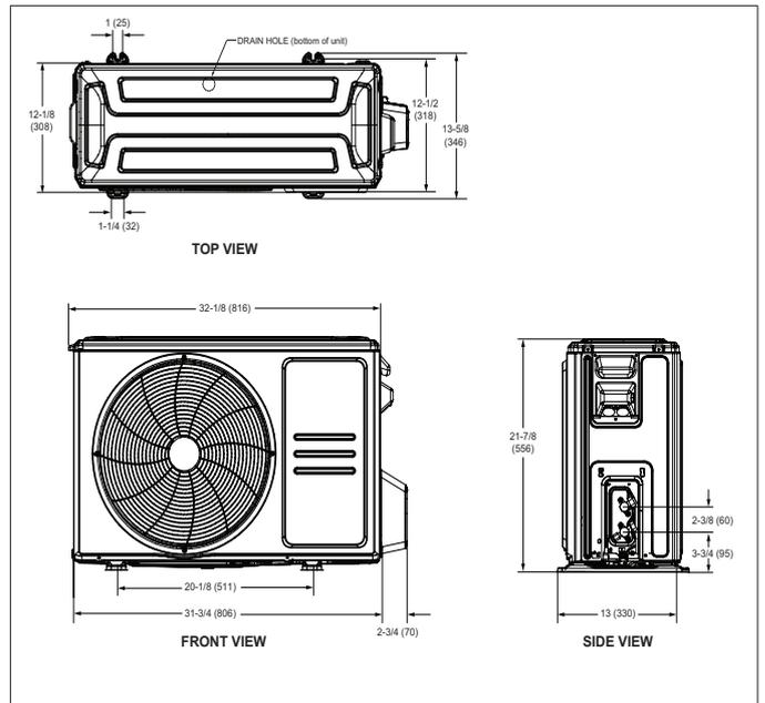
Figure 3. 18K Outdoor Unit Dimensions - Inches (mm)
