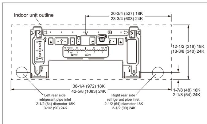
Figure 7. 18K and 24K Indoor Unit Wall Plate Dimensions - Inches (mm)
