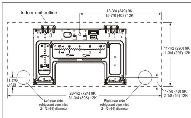
Figure 6. 9K and 12K Indoor Unit Wall Plate Dimensions - Inches (mm)
