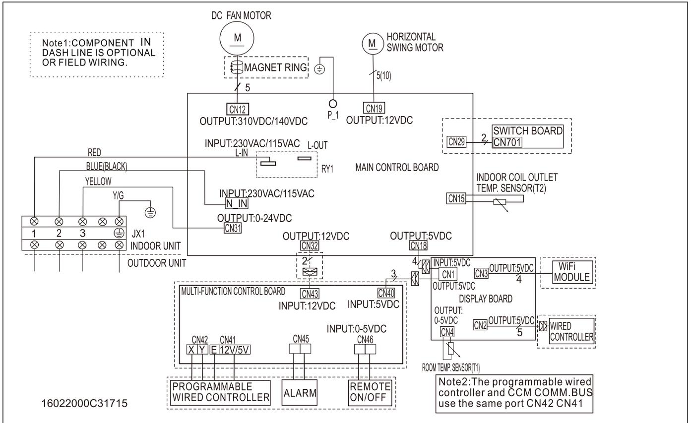
Figure 34. MWHB 09K, 12K, and 18K - 115V and 208/230VAC Indoor Unit Wiring Diagram
