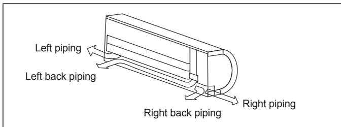
**Figure 11. Determining Exit Locations**
