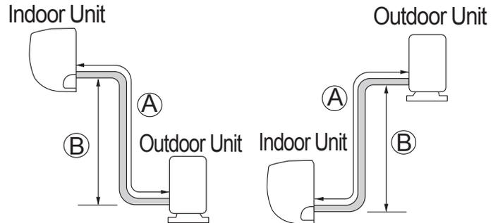
Table 32: Single Zone High Efficiency Refrigerant Piping System Limitations.
