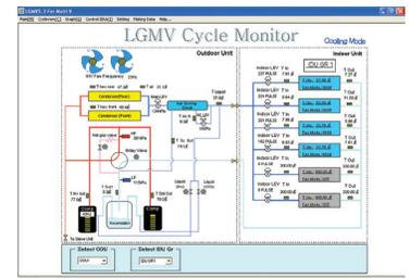
In lieu of connecting to the outdoor unit, user has the option to connect to the indoor unit with the use of a USB to RS-485 connector kit. When connected through the indoor unit, user will not be able to record data.
