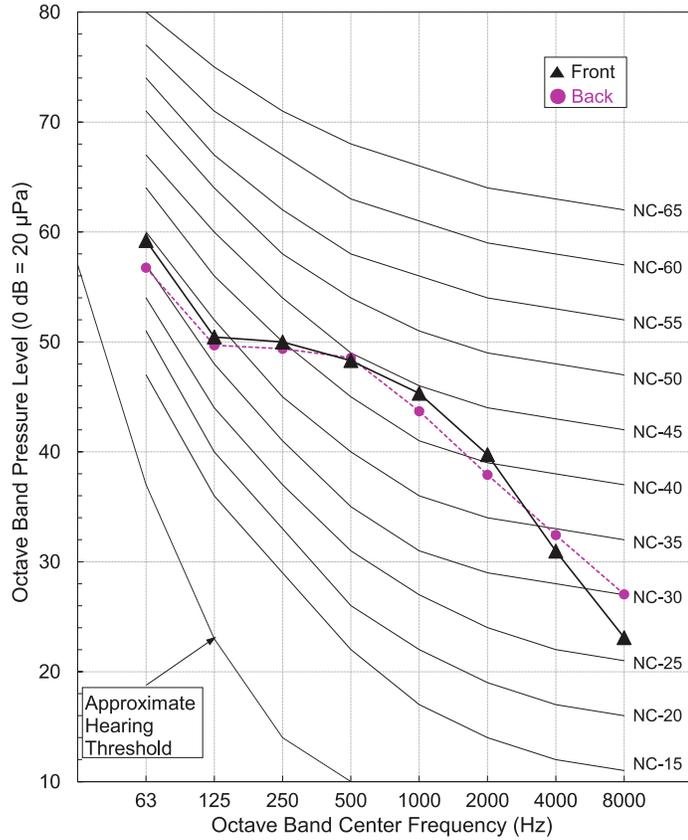
Figure 16: LSU181HSV5 Heating Sound Pressure Level Diagram.
