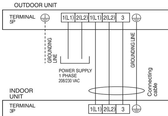
Figure 25: LS181HSV5 System Electrical Connections.
