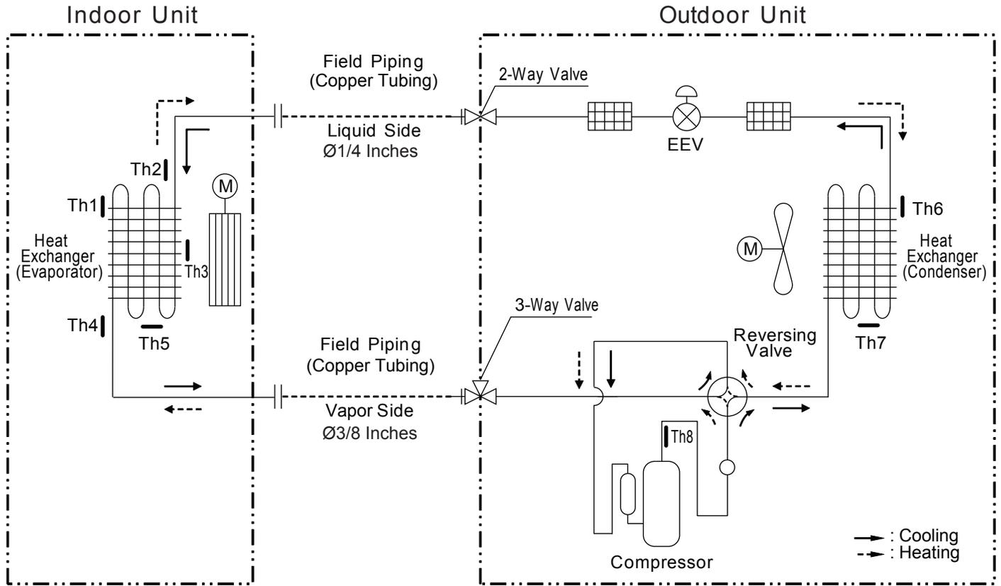
Table 8: Single Zone High Efficiency LSN/LSU090-120HSV5 Thermistor Details.
