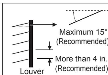
Figure 41: Using “S” Type Louvers.
