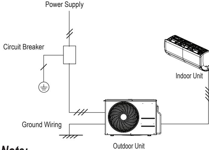
Figure 23: LS181HSV5 General Power / Communications System Schematic.
