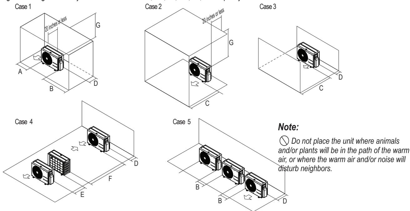
Table 31: Single Zone High Efficiency Wall Mount 9,000, 12,000, 18,000 Outdoor Unit Service Access and Allowable Clearances Diagram Legend.
